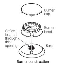
B. Using a 7 mm or 9/32" nut driver, remove the top burner orifices. These may be accessed through the burner opening in the base.
