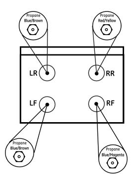
To prevent leakage, make sure the orifices are securely screwed into the gas supply tubes.
